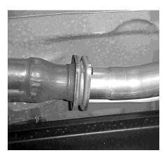
TO REMOVE STOCK EXHAUST UNBOLT THE STOCK EXHAUST AT THE FLANGE BEHIND THE Y-PIPE AND REMOVE. MAKE SURE TO LEAVE ALL RUBBER GROMMETS IN THE FACTORY LOCATION. **YOU WILL RE-USE STOCK NUTS AND BOLTS.** FOR EASIER REMOVAL OF EXHAUST, CUT BEHIND THE MUFFLER. USE WD-40 TO REMOVE HANGERS FROM GROMMETS.
