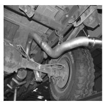
INSTALL OVERAXLE TAILPIPE #C INTO THE OUTLET OF THE MUFFLER 1 1/2" TO 2" USING CLAMP #E TO SECURE PIPE TO MUFFLER. INSERT WELDED HANGER INTO RUBBER GROMMET.
